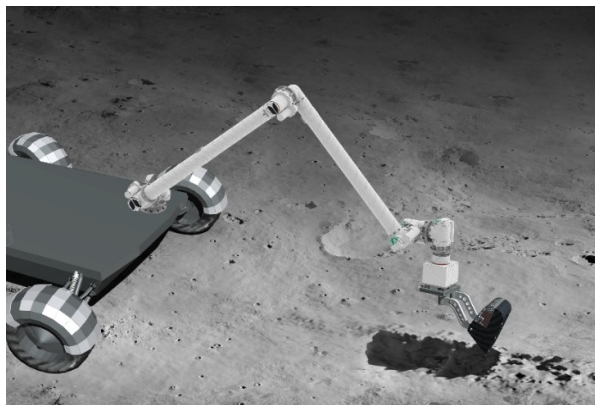
Fig 1: Image of LERA demonstrating trenching capabilities
